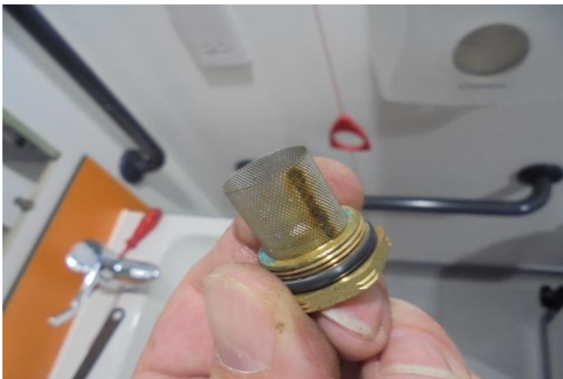
Significant Oxidation Contamination on Contour In-line Strainer
