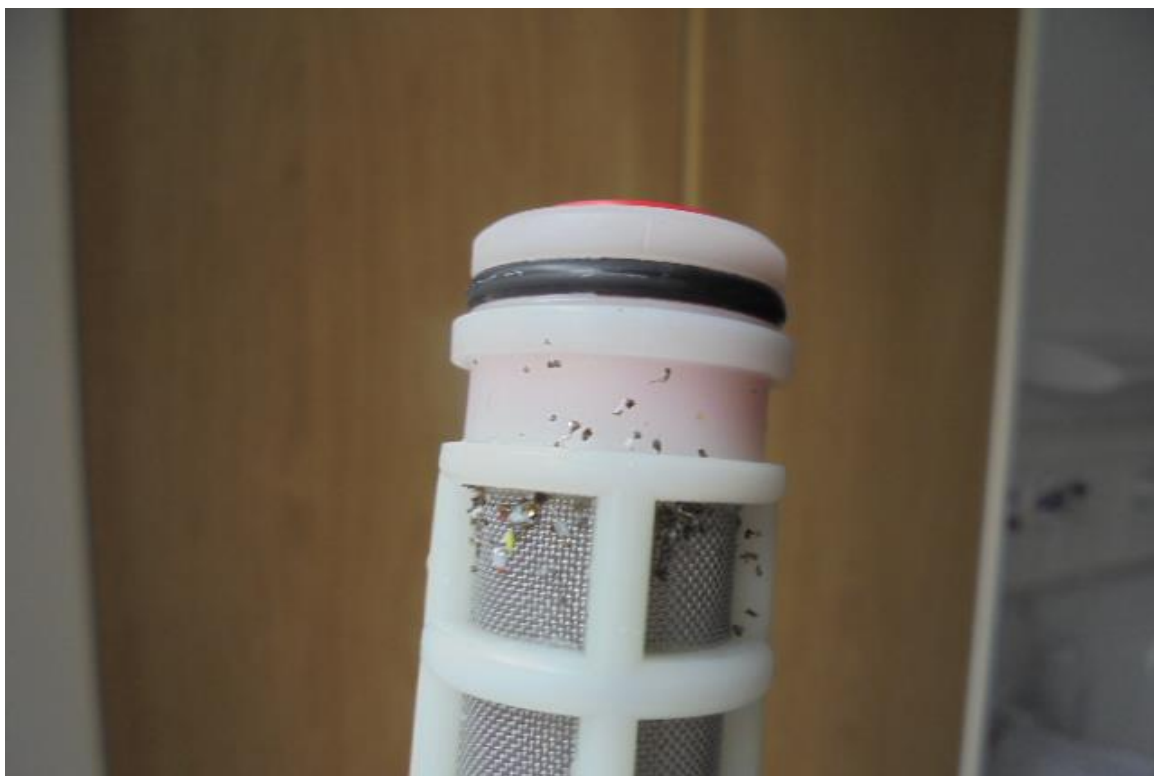
Installation Debris Accumulation on Markwik Inlet Filter
