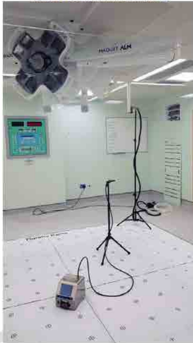
Figure 14 UCV entrainment test setup
