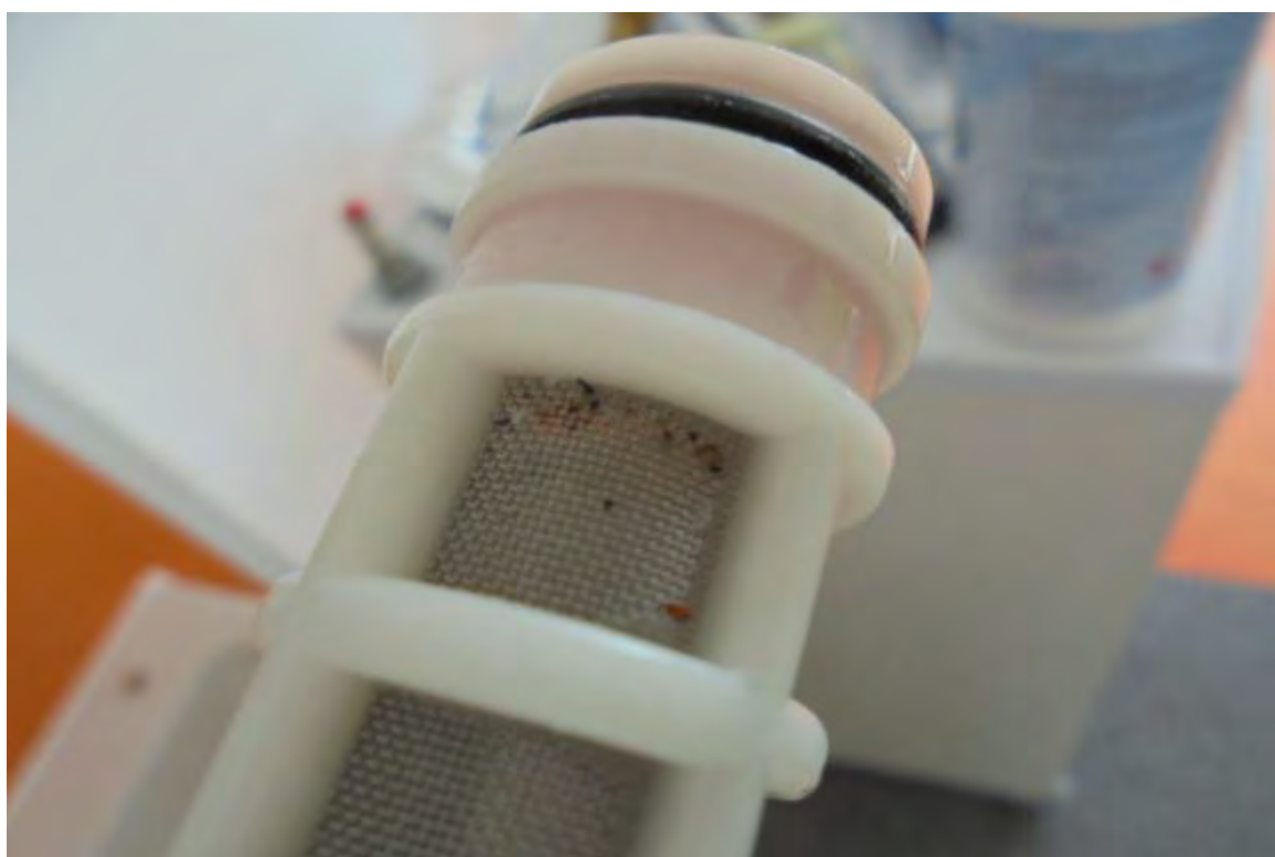
Further Illustration of Minor Particulate Accumulation on Markwik Inlet Filter
