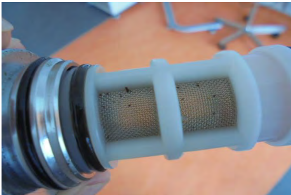
Illustration of Slight Particulate Accumulation on Markwik Inlet Strainer
