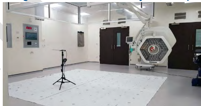
Figure 13: UCV 1m air velocity test set-up
