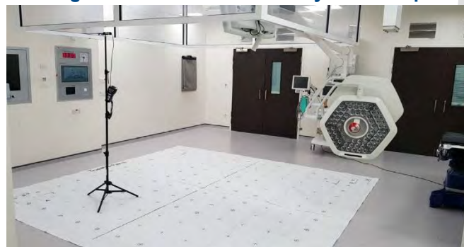
Figure 12: UCV 2m air velocity test set-up
